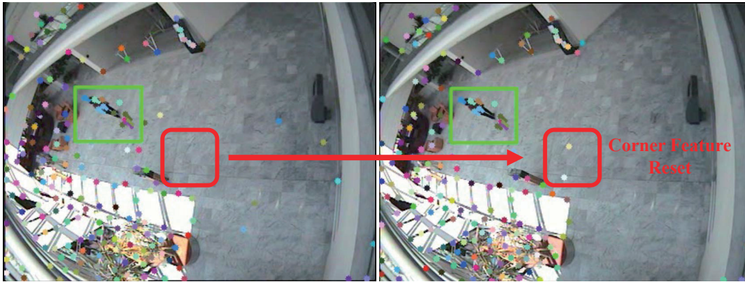
Figure 3.2: Example of corner feature reset method.
