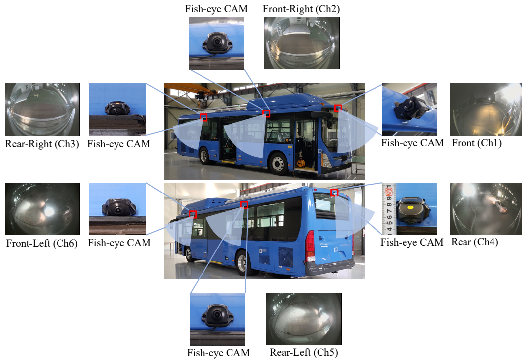
Figure 4.2: Fisheye cameras settings mounted on a hydrogen-powered bus; six fisheye cameras were used to collect the surrounding images.
