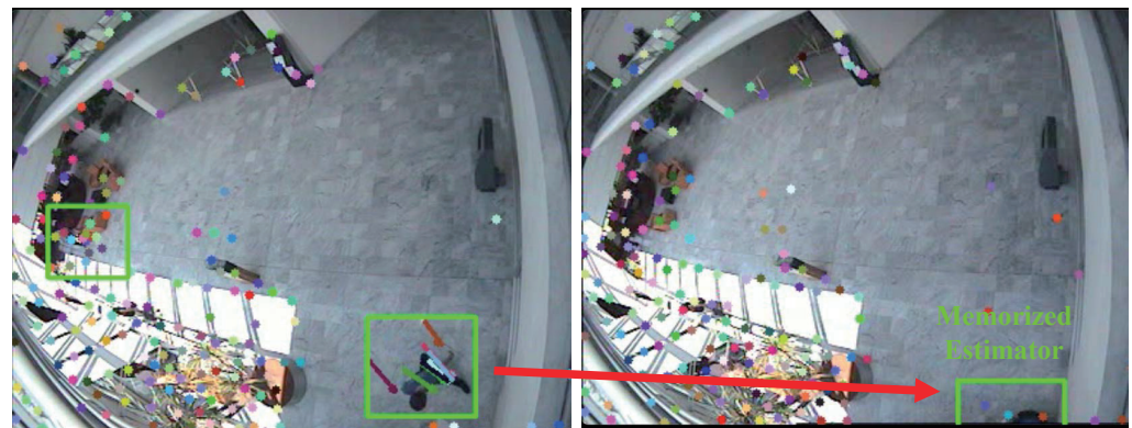
Figure 4. Example of the memorized estimator method. The green boxes show detection of moving objects. The green detected box is maintained on the target over a given time span.
